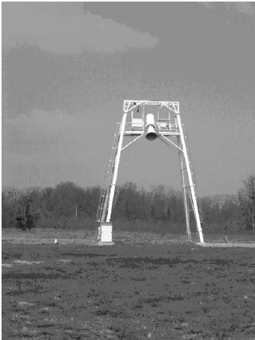
Fig. 1. LEWIS on its supporting structure and with rotating mechanism. The rotation axis is 13.6 m high. The length of LEWIS is 3 m, and the weight is about 200 kg.
