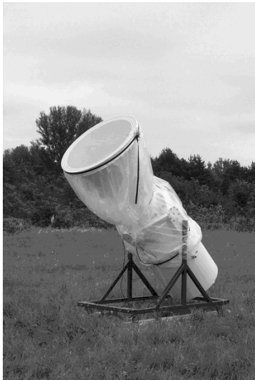
Fig. 11. Overall calibration using the sky. The plastic foil was implemented to protect the instrument (always pointing toward the sky for several months) so as to avoid collecting rain through the horn. Specific measurements showed that as long as the plastic did not fill up with a significant amount of water, and as long as water did not gather in small top-to-bottom rivulets, the impact of this improvised radome could not be measured in the collected data.
